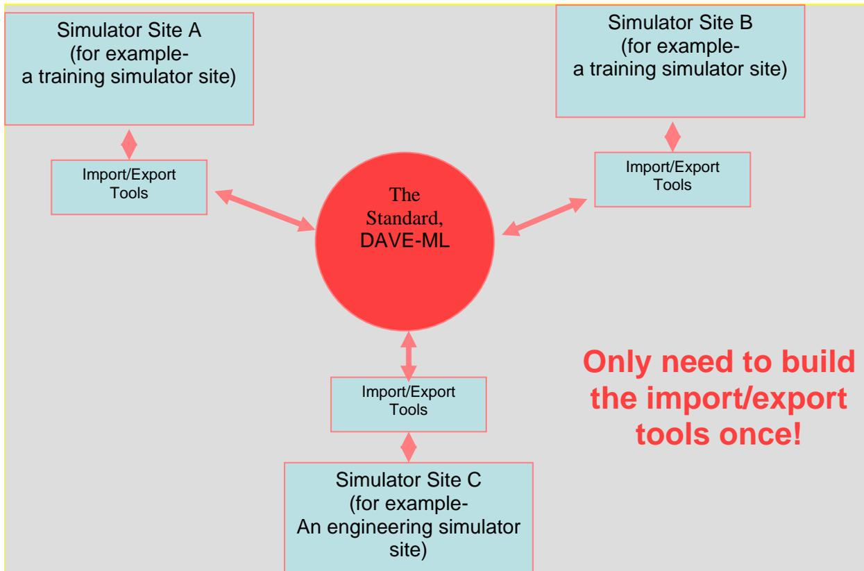
Figure 1. A Standard Format for Exchanging Simulation Modeling Data Between Simulation Facilities
